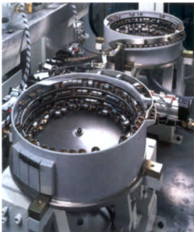
In this application, bowl feeders drop bushings into place, where they are automatically inserted into castings. Pick-and-place units transfer the castings into and out of the station.
